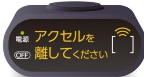
Device to prevent unintended acceleration from pedal misapplication: in-vehicle indicator
