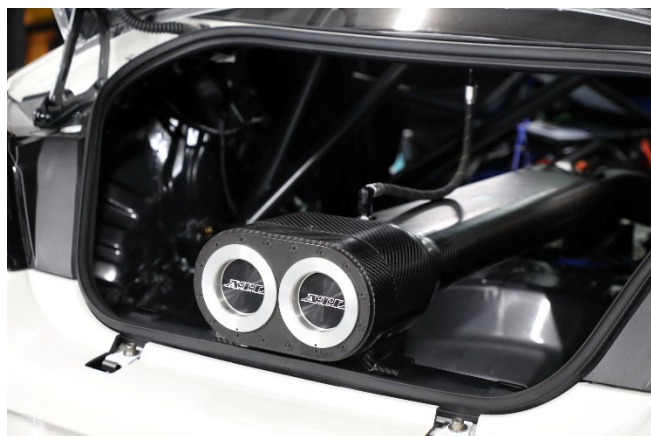
Team SDA Engineering BRZ CNF Concept Fuel Supplying System
