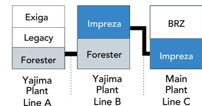
Bridge production of the Impreza and Forester models serves as a kind of control valve, allowing the lines to respond flexibly to demand for each model and maximize the utilization of production capacity.
