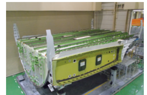
Center wing box manufactured at the Handa Plant
