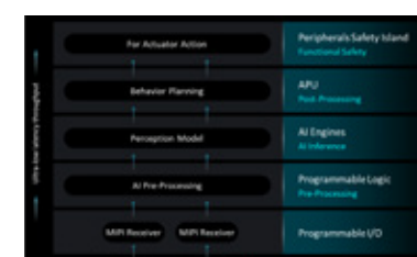
Workflow of stereo image data processing (From AMD's Keynote at Embedded World 2024)
