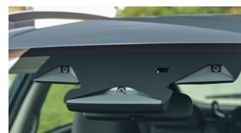
New-generation EyeSight stereo camera + wide-angle single lens camera
