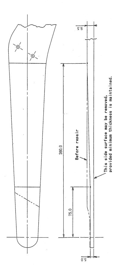
FIGURE 1 REPAIR LIMITS - FA-200 INBOARD FLAP HINGE FITTING
