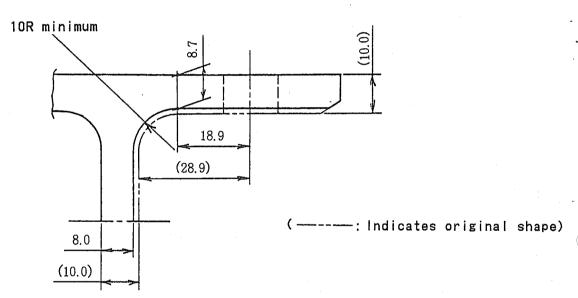
Dimensions show repair limits; The dimensions given in parentheses are the original dimensions.
