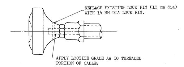
These improvements have increased locking strength greatly (approximately three times), thus eliminating possible failure of the lock pin which can be attributed to overtightening. It is, therefore, recommended that the cable assy be repaired in accordance with the following procedures, if failure of the lock pin occurs.
