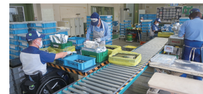
The height of automatic door switches and work stations is set at a level that is convenient for those using wheelchairs
