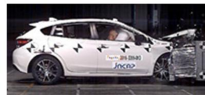
Image of Impreza JNCAP\* Frontal Offset Crash Test
