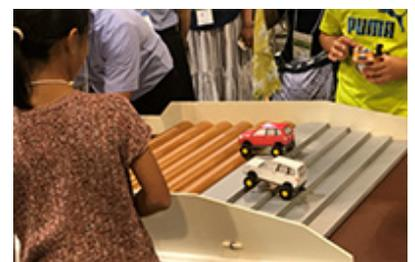
Experiment to see the difference between four and two wheel drives
