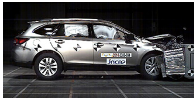
Image of Legacy Outback JNCAP Frontal Offset Crash Test Photo courtesy of the National Agency for Automotive Safety & Victim' s Aid (NASVA)
