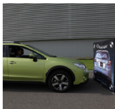
EyeSight active driving assist system employing stereo camera.
