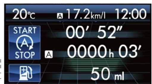
The engine's total stop time and fuel savings are displayed on the multifunction display
