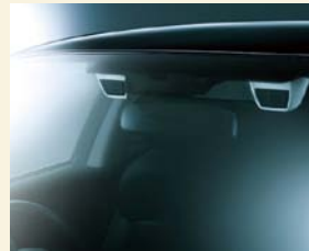
Estimating the distance to a vehicle ahead with two cameras, which function like human eyes
