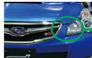
An example of the material indication: "PP" means polypropylene
