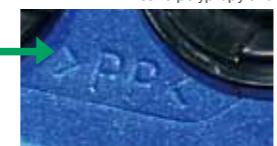
An example of the material indication: "PP" means polypropylene
