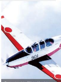
The new primary trainer T-7 being delivered since the fiscal 2000 has improved performance and noise level by employing a turboprop engine over the preceding trainer. It also has better interior comfort with a newly installed air-conditioning unit and more space in the cockpit.
