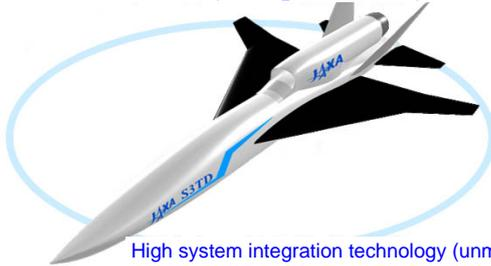
High system integration technology (unmanned aircraft technology for autonomous flights from take-off to supersonic cruising and landing)
