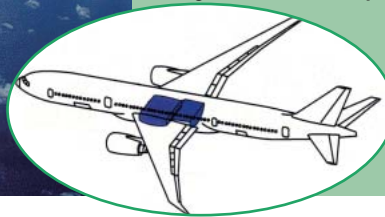
(Below) Blue portion: the Center Wing section where FHI Aerospace Company is responsible for development.
