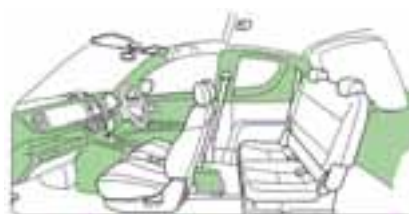
Green parts: Integrated materials are used in these parts.
