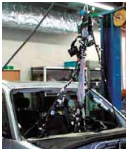
Picture 1 : Wire harness dismantling experiment
