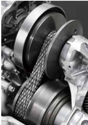
Lineartronic: a new developed CVT(Continuously Variable Transmission)
